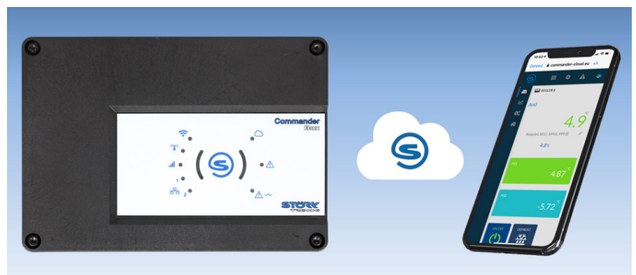
Figure 1: Connection from the controller to the cloud via the Commander Box
