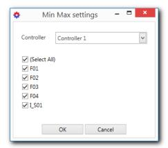
Select the respective controller in the dropdown box and set the checkmarks for the desired measured values.
